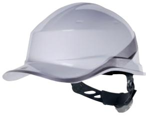
ABS safety helmet. Innovative "baseball cap" shape to improve vision when looking up. Also tested for front to back wearing, to reduce encumbrance. Polyamide cradle: 3 textile straps with 8 fixing points. Foam sweat band. Innovative button adjustment "colour to colour" for head size 53 to 63 cm. 2 possible positions of the headband (top/low) for a better comfort. Electrical insulation up to 1 000 V.A.C. or 1 500 V.D.C.
