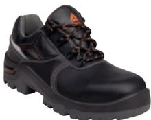
Upper: Pigmented split leather, S3 water resistant treatment. Lining: Polyamide mesh. Insock: Removable premolded - Polyamide on EVA. Outsole: Injected - PU bi-density. Non metallic footwear.
