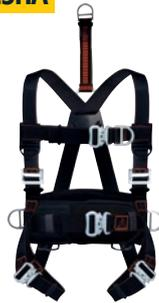
Harness with positioning belt. 2 fall arrest anchorage points (dorsal - sternal). 6 adjustable buckles including 4 automatic. Positioning belt with thermoformed. 2 lateral work positioning anchorage points. 1 extension lanyard.
