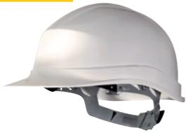
UV-resistant high density polyethylene (HDPE) or polypropylene (PP) safety helmet. Low density (LDPE) polyethylene cradle with 8 fixing points. Sweat band. Manual adjustment: head sizes 53/63 cm. Electrical insulation up to 1 000 V.A.C. or 1 500 V.D.C. Standard holes for accessories. Anchorage for chin straps with 2 or 4 points.
