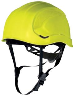
ABS safety helmet. Mountain helmet style: without visor for the best vertical vision. Less encumbrance. Light. Polyamide cradle: 3 textile bands with 8 fixing points. Thermoformed sweat band. Innovative adjustable ROTOR system: head sizes 53 to 63 cm. Sold with 3 point chin strap. Specially designed for working at height. Electrical insulation up to 1 000 V.A.C. or 1 500 V.D.C.
