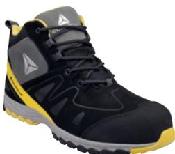
Upper: Suede split leather (cowhide), S3 water resistant treatment with front rubber reinforcement. Lining: Polyester non-woven and knitted mesh. Insock: Removable premolded - Polyester on EVA. Outsole: Cemented - Phylon. Outsole: Rubber. Non metallic shoe.
