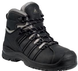
Upper: Full grain leather, S3 water resistant treatment. Lining: DELTA-TEX™ waterproof polyester membrane. Insock: Removable - polyester on EVA. Midsole: Injected - Dual density PU. PU bumper protection. Non metallic footwear.
