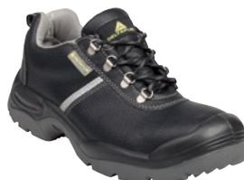
Upper: Pigmented split leather, S3 water resistant treatment. Lining: Polyamide. Insock: Removable premolded - Polyamide on EVA. Outsole: Injected - Dual-density PU with bump cap.
