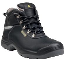
Upper: Pigmented split leather, S3 water resistant treatment. Lining: Polyamide. Insock: Removable premolded - Polyamide on EVA. Outsole: Injected - Dual-density PU with bump cap..
