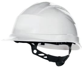
UV-resistant high density polypropylene (PP) safety helmet. Polyamide cradle: 3 textile bands with 8 fixing points. Foam sweat band. Innovative adjustable ROTOR system: head sizes 53/63 cm. 2 possible positions of the headband (high/low) for better comfort. Electrical insulation up to 1 000 V.A.C. or 1 500 V.D.C.
