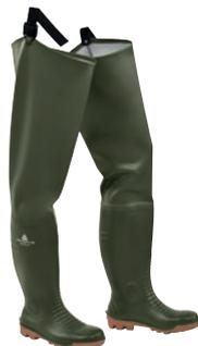
Coated canvas: PVC, height: 80 cm. 100% waterproof high frequency heat seal. Lining: cotton jersey. Nylon retaining straps. Protection of the malleoli. Rear removal lug. Protective toe cap: stainless steel. Anti-perforation mid sole: stainless steel. Sole: PVC - Nitrile with large cleats.
