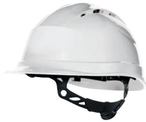
Ventilated UV-resistant high density polypropylene (PP) safety helmet. Polyamide cradle: 3 textile bands with 8 fixing points. Foam sweat band. Innovative adjustable ROTOR system: head sizes 53/63 cm. 2 possible positions of the headband (high/low) for better comfort.
