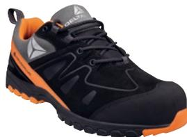
Upper: Suede split leather (cowhide), S3 water resistant treatment with front rubber reinforcement. Lining: Polyester non-woven and knitted mesh. Insock: Removable premolded - Polyester on EVA. Outsole: Cemented - Phylon. Outsole: Rubber. Non metallic shoe.
