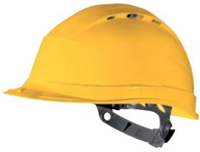
Ventilated UV-resistant high density polypropylene (PP) safety helmet. Polyethylene cradle: 8 fixing points. Sweat band. Manual adjustment: head sizes 53/63 cm. 2 possible positions of the headband (high/low) for better comfort. Helmet with adjustable ventilation.
